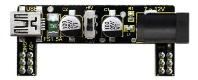
Keyestudio breadboard power module is compatible with 5V and 3.3V, suitable for MB102 breadboard. This module includes dual independent control, one can be powered by USB port to output the voltage constantly for DC 5V; Another one is to power with DC 6.5-12V, and output controlled by dial switch, respectively for DC5V and DC3.3V.
