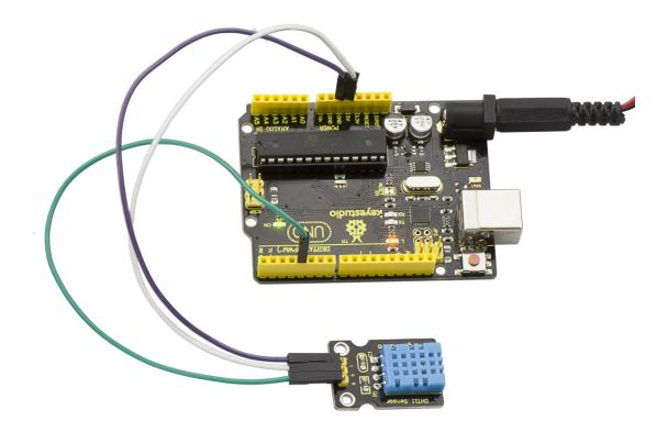
Then open the serial monitor and set the baud rate to 9600, you will see the current temperature and humidity value.
