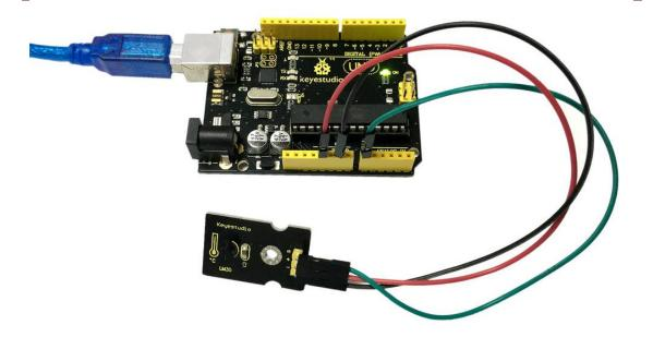
Upload well the code to the board, then open the serial monitor and set the baud rate to 9600. You will see the current temperature value shown below. The value may be slight difference due to different places and weather.
