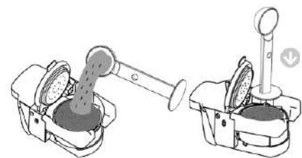
8. Insert the adapter (5) in the adapter input on the appliance.
