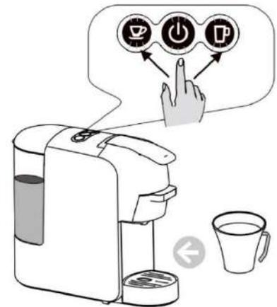
14. When the brewing procedure is complete, press On/Off button to turn off the appliance.
