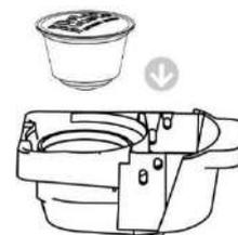
8. Insert the adapter (5) in the adapter input on the appliance.
